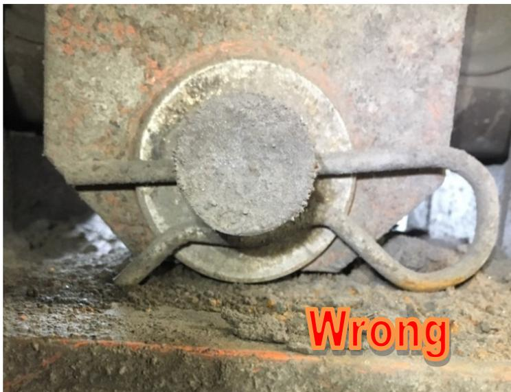
Cleanliness: It is important to keep the load cells area reasonably clean. Build-up of detritus as shown here can affect accuracy if the deposit hardens (Lime Dust can set like concrete) and limits the deflection of the load cell.
