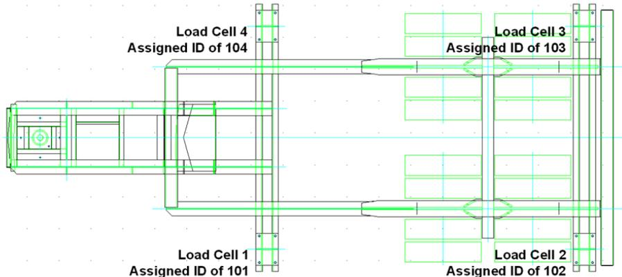
All load cells returned from the factory, whether new or refurbished, will be supplied with an ID of 1 and so the load cell will need to be reprogrammed with the ID corresponding to the position on the trailer where it will be located.
