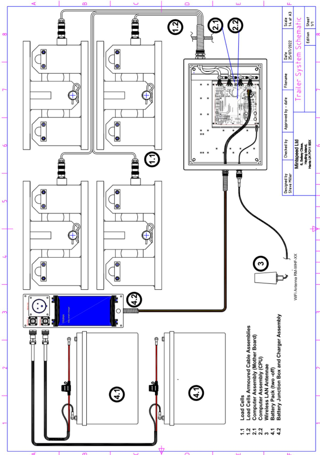
The ScrapMan computer assembly showing the external connections for; Load Cells, Power and WiFi Antenna
