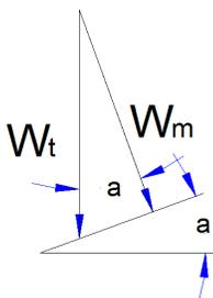
e.g. A precise dead weight of 100.00T would, at 5° be measured at 99.62T, if during calibration the full scale deflection was then set at 100.00T, all subsequent measurements would be out by 0.4% (unless measured on the same slope). This means that all loads would need an extra 0.4% of material to reach a specified target thus using more stock.
