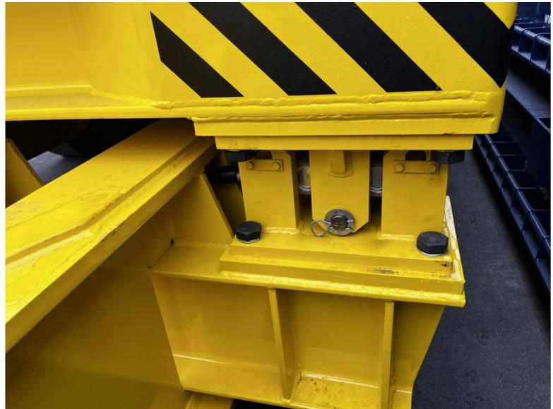
**N.B. It is good practice to periodically clean the load cells from any debris. Any build-up of detritus that affects the deflection of the load cell **will also affect the accuracy.****
