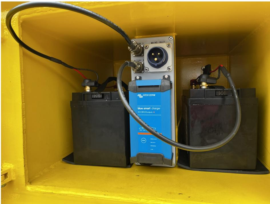
The batteries can be *Hot Swapped*; it is **not** necessary to turn the computer off when changing but if both are changed at the same time, the computer will perform a Power OFF/ON RESET when powered up again.
