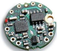
Each load cell and its associated **D-Cell** are irrevocably tied together during factory calibration with settings of **zero load** to **Full Scale Deflection** (depending on the Trailer Load Rating) in 10Kg increments) retained in the non-volatile memory. Consequently, they are effectively **digital** in that no additional calibration or scaling should be required on installation or replacement.
