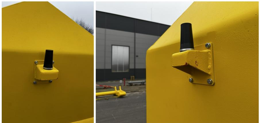
The Antenna is designed to operate in the open air at **2.4GHZ** and is mounted to a bracket at the very front of the trailer roof; this is the safest place for the antenna but inevitably some will get broken. The antenna screws into the base as shown in the photographs. The base is complete with a coaxial cable 2m long that runs from the underside of the bracket to the computer enclosure where it terminates in a "N" type connector.
