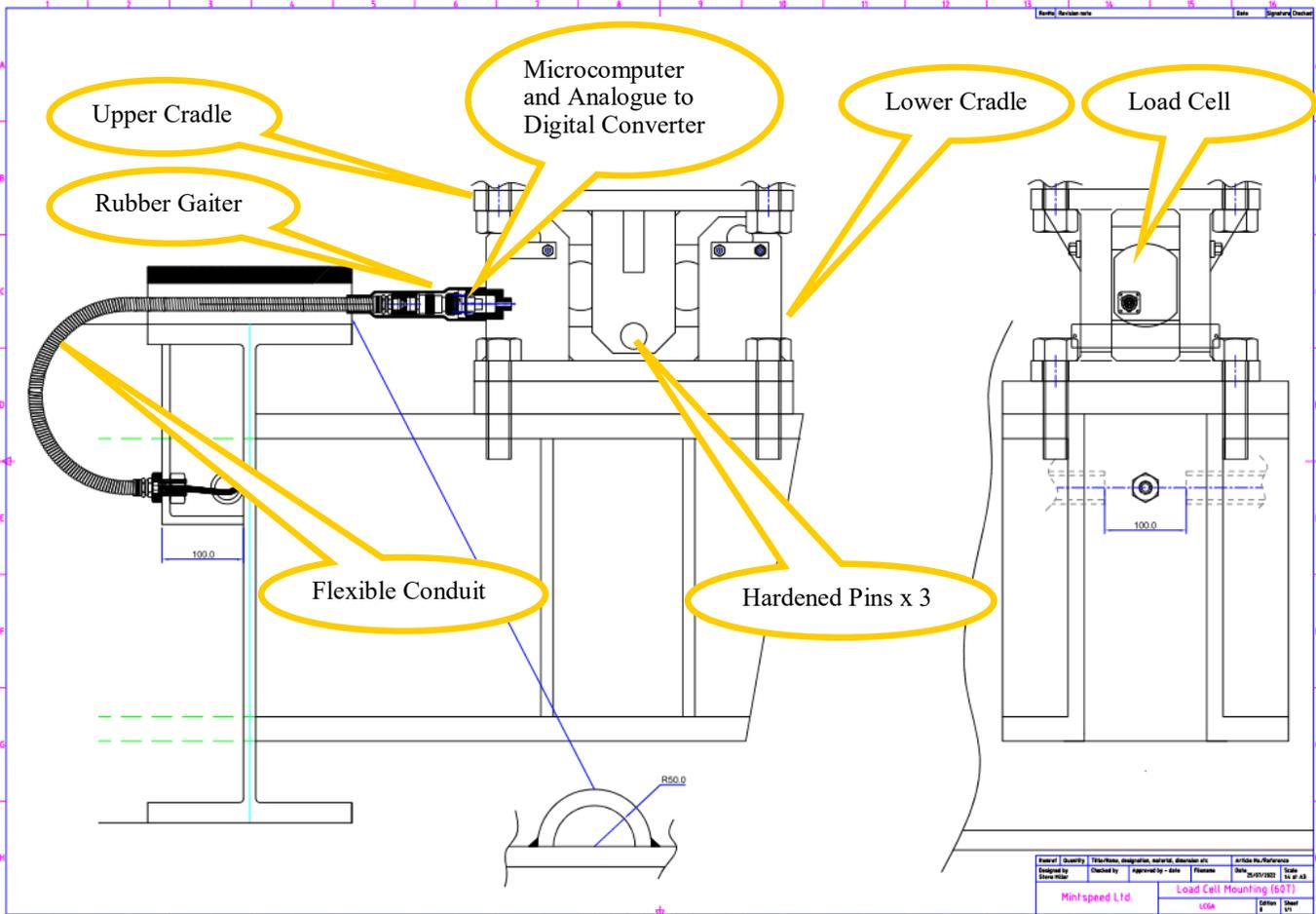
The **D-Cell** (shown below) is very small microcomputer housed in the machined, stainless steel cylindrical enclosure at the inboard end of the load cell, this **D-Cell** module includes the following functionality;
