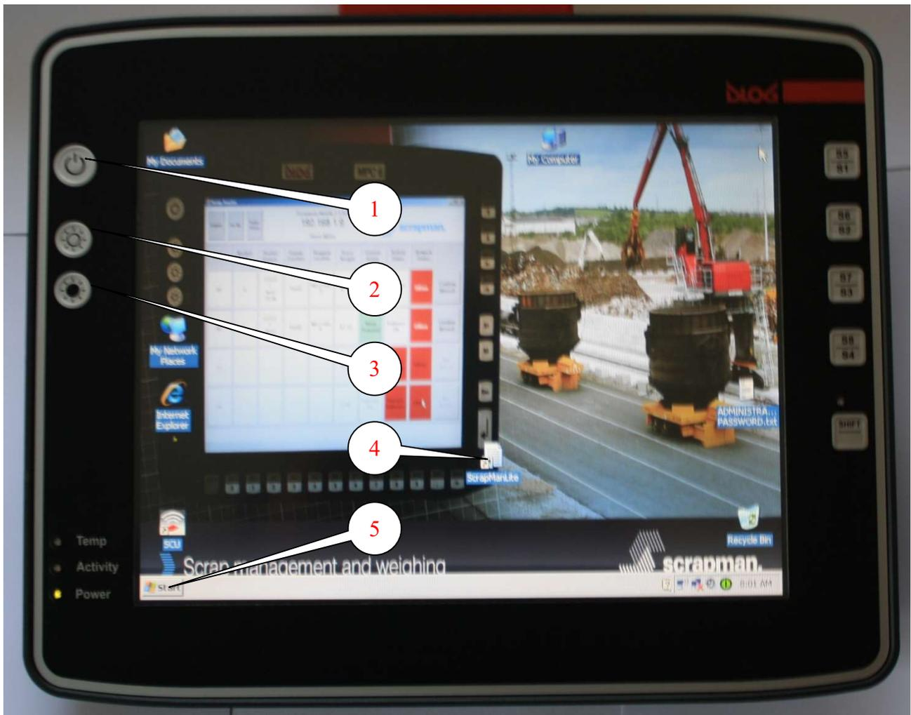
The computer is connected to the ignition circuit and if the ignition is turned OFF, the computer will commence an automatic shut-down sequence with a 5 minute count-down; this can be adjusted and is explained in the D-Log Manual.
