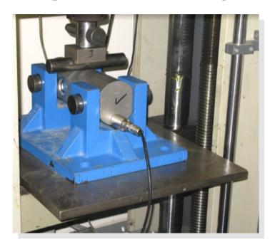
Load Cell under test and calibration in a hydraulic Test Rig.
