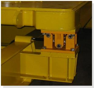
Load Cell complete with mounting cradle in-situ on Trailer Chassis
