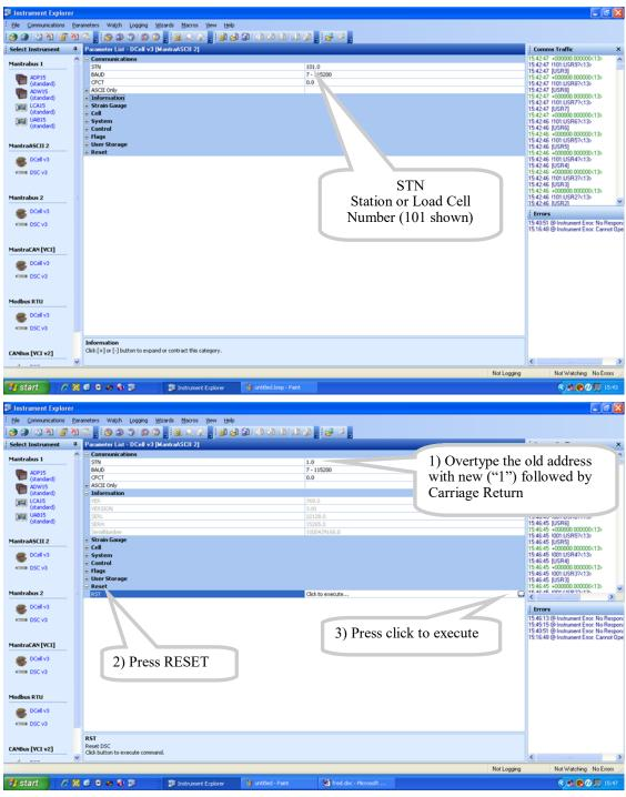
This should have changed the address; as a check, repeat the procedure using the new address of "1" at the opening screen to see it has been accepted.
