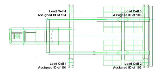
Any subsequent change of any load cell requires the ID of that load cell to be **EITHER** set to the correct ID for that position (eg *103* for rear, RH side) **OR** set to "1" which will force the system to reassign an ID automatically (*103* in the case of rear, RH Side).
